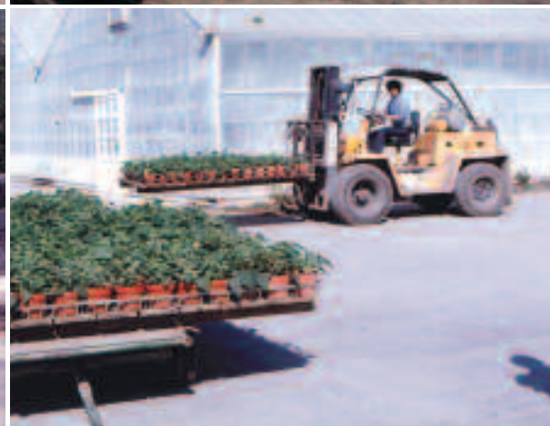
Top left: Wood, plastic and cardboard are used for pallets that hold the materials growers receive. Top right: This low-cost, hand-powered pallet truck rolls easily on a concrete floor. Middle left: A battery-powered pallet truck will move large loads over long distances. Middle right: Three-point hitch pallet forks will lift and carry heavy loads easily. Bottom left: An articulated fork lift makes loading carts easy in confined areas. Bottom right: Extension forks are needed to handle large trays. (Photos courtesy of John Bartok)
